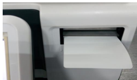
⑧ Press the feed button, the label is printed out
