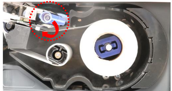
⑥ Insert the cassette and turn the lever to the closed position
