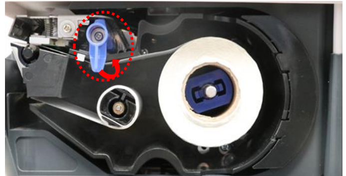
② Turn the lever to the open position
