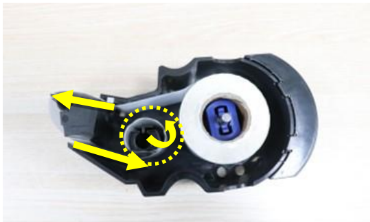
⑤ Insert a new label roll, then insert the backing paper under the slot in the reel and close the fixing lever
